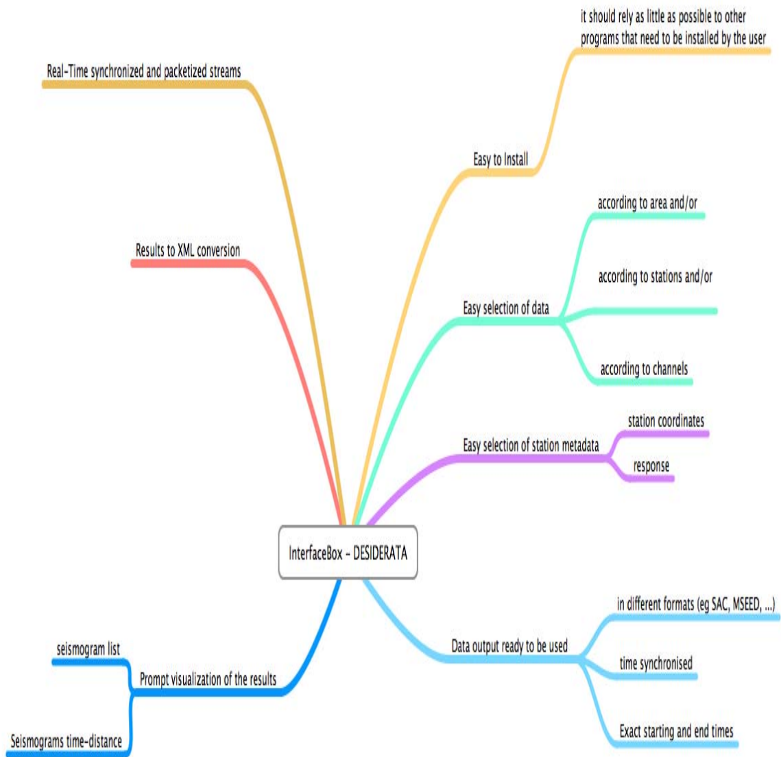
Figure 6. Simplified cartoon illustrating some basic wishes of the seismological community for what concerns data access and basic analysis.
